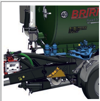
Hydraulic displacement forced steering
