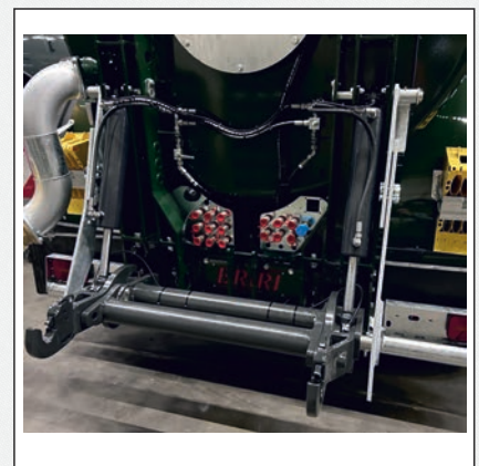
Hoist 5 tons with pendulum compensation
